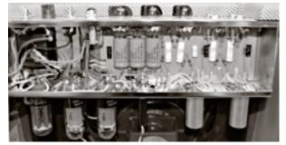
just grounded one leg of the 6.3V to the chassis, (to use it as one side of the filament), and ran one wire to the other side of the filaments. We use the same wire routing, the same construction techniques with brass eyelets, all carbon comp Allen Bradley resistors, Carling switches, and the tube sockets are NOS made for the military in 1952.
